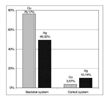
Fig. 4. Percentage of Cu and Ag extracted from ore after 35 days autotrophic bioleaching in tube bioreactors
