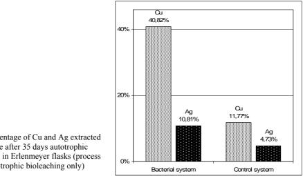
Fig. 1. Percentage of Cu and Ag extracted from ore after 35 days autotrophic bioleaching in Erlenmeyer flasks (process 1: autotrophic bioleaching only)
